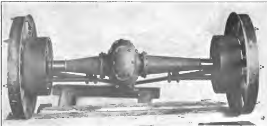
Fig. 3—Rear axle construction, showing a steel shell; large brakedrums and a stout bridge
